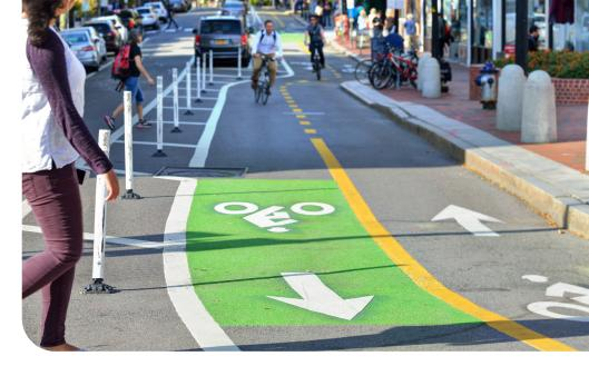
the bike lane, cyclist speeds often vary greatly and thus ample space for passing is needed, and the potential for an increasing the likelihood of cyclist on cyclist collisions especially if ample space for passing other cyclists is not provided.
