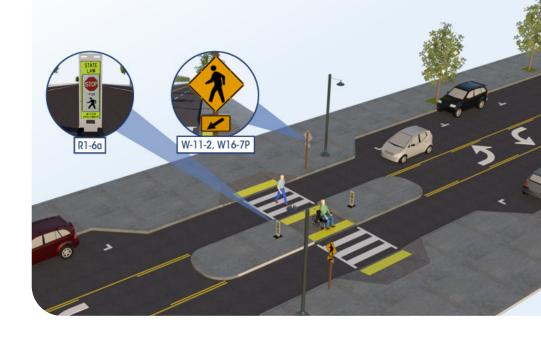
realigns roadways and intersections increasing safety for all roadway users. Crosswalks and other bicycle and pedestrian facilities should be reconstructed and striped. The construction of this extended curb can often shorten the distance for pedestrian crossings, create right-angle intersections, and reduce roadway pavement (and associated maintenance).
